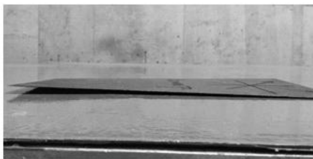
Fig. 13. A warped CFRP
