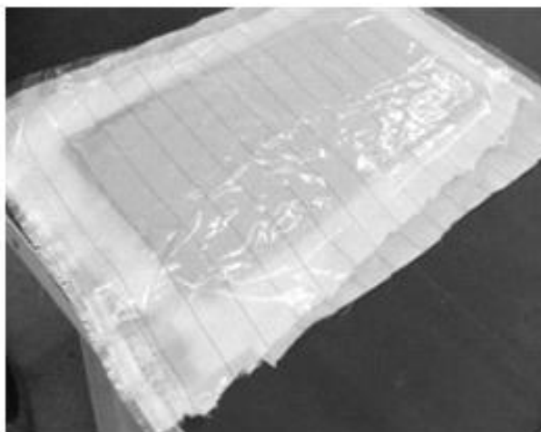
Fig. 12. A manually cut Carbon being covered with a resin material before curing at the Center of Composite Technology, Kazan, Russia
